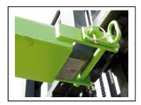
The vertical pin system reduces the risk of the pin being removed, even when it is damaged by striking the ground. With the pin located in a vertical location the bottom of the pin may be damaged, but this will result in the pin being bent and not removed.
