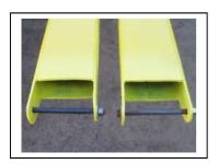
The fork extension retaining pin should be a bolted system which allows the retaining pin (bolt) to be secured with a spanner, removing the risk that contact with the ground can remove pins and enable the pins to come loose / off.
